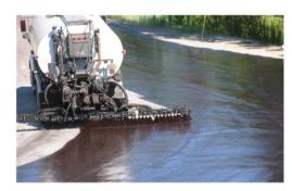
Due to their environmental, technical, economical, and application advantages; bitumen emulsions are extremely suitable substances for all kinds of applications. Phoenix International A/S produces all kinds of cationic, anionic, and polymeric bitumen emulsions for different purposes. Special emulsions such as: Tack Coat, Prime Coat, Fog Seal Chip Seal, Slurry Seal, Micro Surfacing, Road Mix and Cold Mix.
